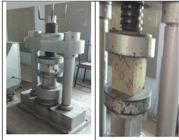
Figure 2 Compressive strength test of (0.5%PPF+0.1%) HFRC
