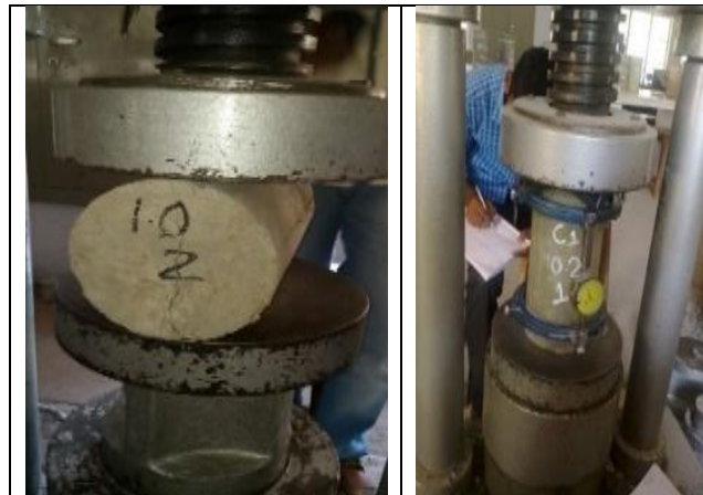
Figure 1 Stress strain test for (0.2%PPF+1.0%) HFRC
